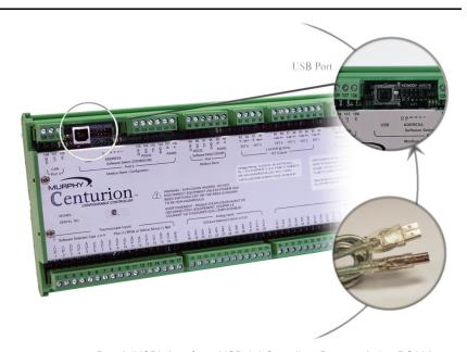
Port 2 (USB): Interface: USB 1.1 Compliant Port emulating RS232 communications via PC driver
