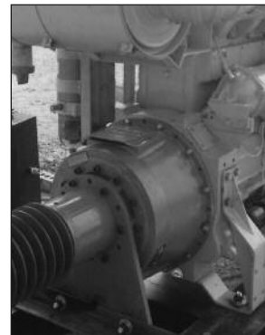
Wichita PTO mounted on Caterpillar diesel engine.
